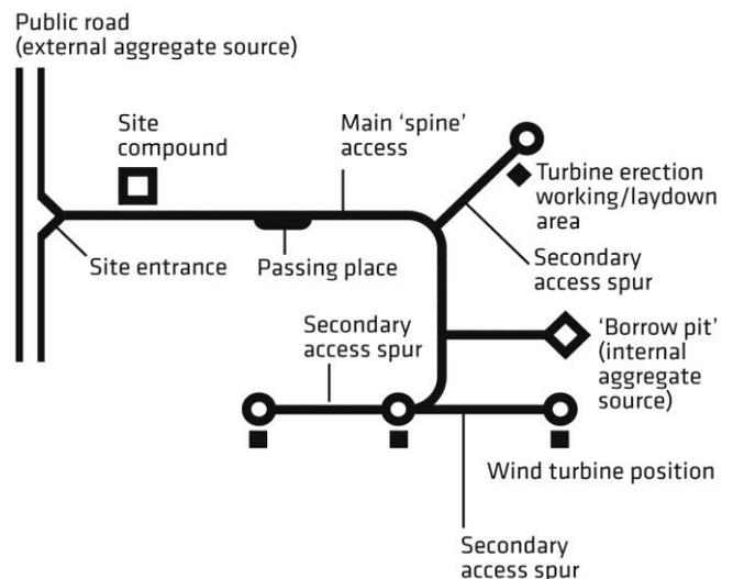
Figure 1: Schematic of the salient features of a wind farm layout
