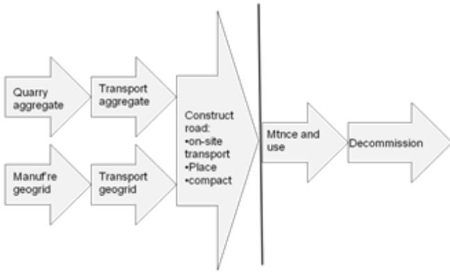
Figure 3: Process map for calculating embodied carbon
