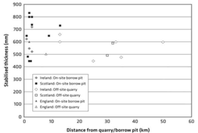
Figure 5: Road thickness v distance from aggregate source
