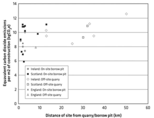
Figure 7: Carbon footprint v distance from fill source
