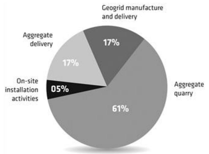
Figure 8: Analysis of the carbon footprint components
