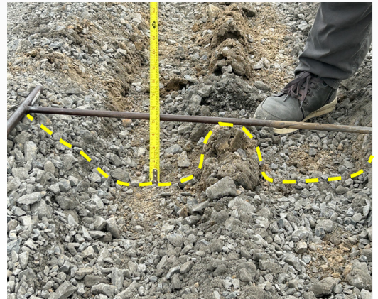
Section 3 - Biaxial Grid 2: 100mm rut
