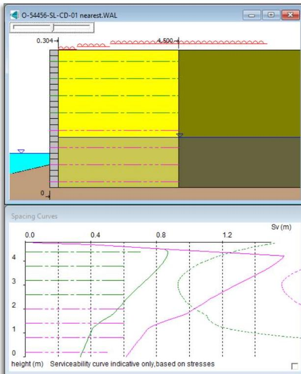
In this case, there is no issue with **TensarSoil**. It is important that surcharge loads are not placed on the top of the facing.
